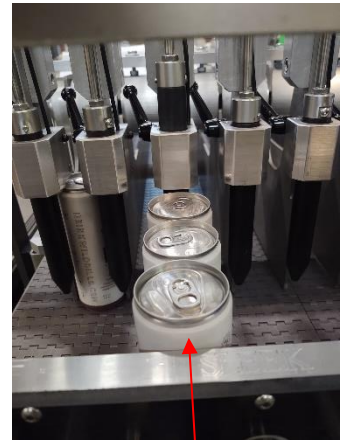
Cans in line with stop pin
