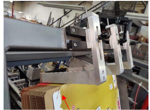
Upper detent arm clearance
